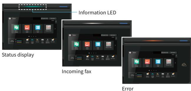
**On-Screen System Information** The control panel shows the state of your MFP, displaying current operation and notifications for things like paper, toner, and maintenance.
